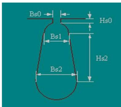
Fig. 2: Stator slot
