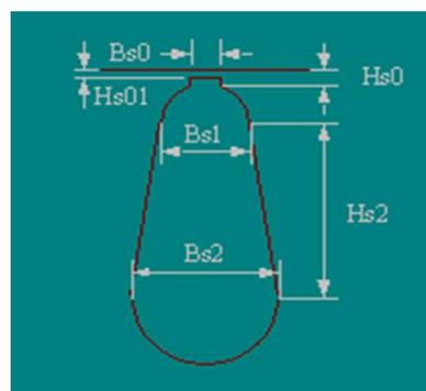
Fig. 3: Rotor slot
