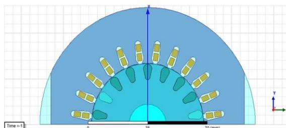
Fig. 4: Overview of stator and rotor slot
