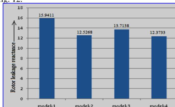
Fig. 12: Bar graph of rotor leakage reactance
