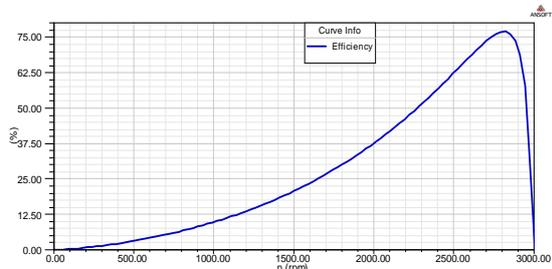
Fig. 6: Curve of efficiency of M19\_24G design
