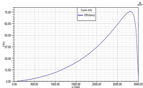
Fig. 5: Curve of efficiency of D23 design
